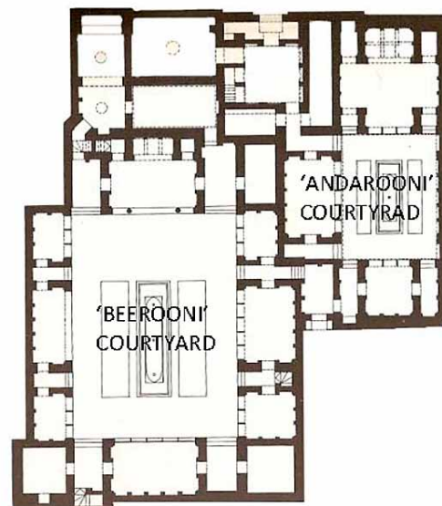
Fig. 6. A plan of a TPH complex with two different 'Andarooni' and 'Beerooni' courtyards in Gazorgah neighborhood in Yazd (Ghezlbash, Abouzia 1985: 38)
