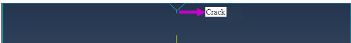
d) Model of notched pre-cracked wire specimen in wire frame
