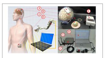
FIGURE 1 | Images of the implantable device. (A) Titanium skull casing. (B) 3D high-density multiple electrodes. (C) Stretchable spiral cable. (D) Data and power management unit. (E) Wireless power supply (transmitter). (F) Wi-Fi access point. (G) ECoG monitoring software. (H) Example of assistant device.
