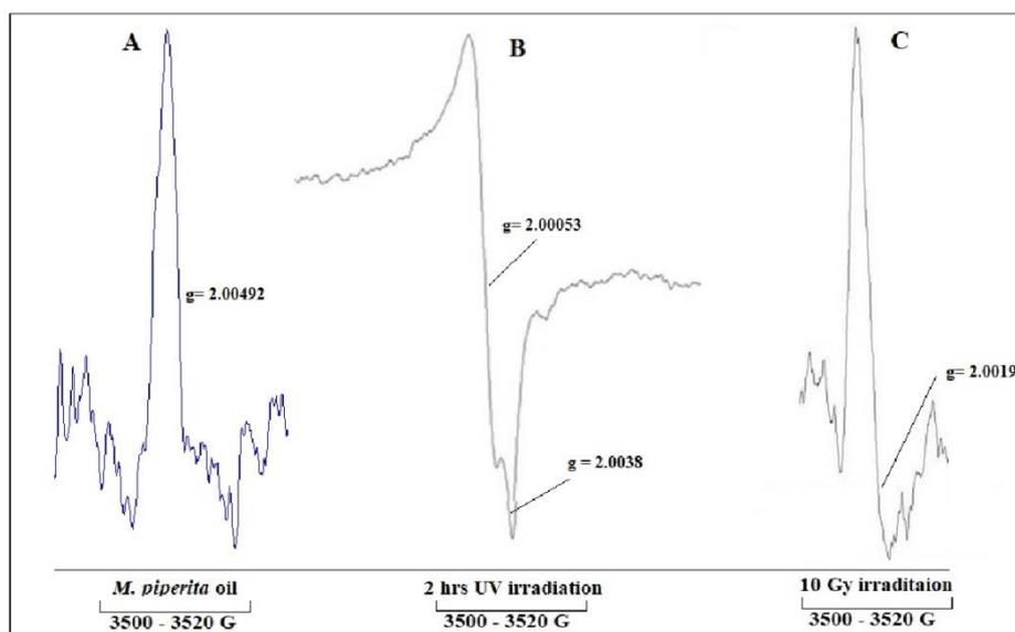
**Figure 6.** First derivative of the absorption curve (arbit. units) of *M. piperita* oil registered before radiation (A) after 2h UVB (B) and 10 Gy irradiation (C) with respect to the applied magnetic field (G).
