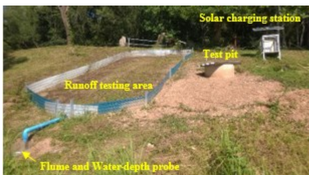
Fig. 3. Picture of the test site showing instrumentations installed.
