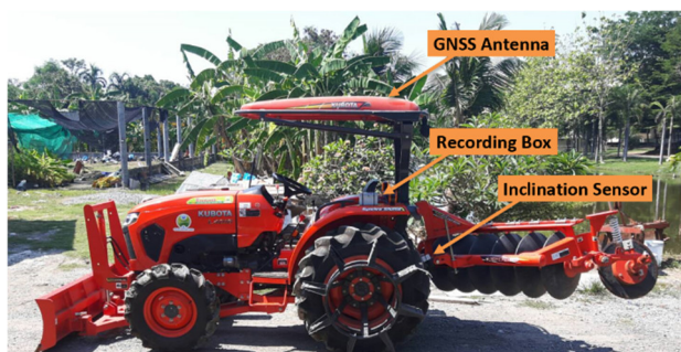
Fig. 2. The test tractor with the instruments installed.
