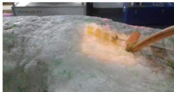
Figure 2. Setup for percentage depth dose measurements on pelvic phantom
