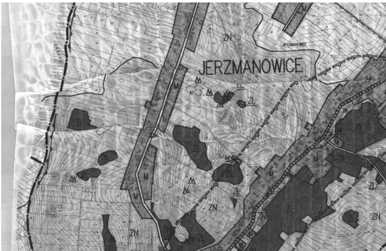
Fig. 2. Deformations of a scanned drawing of the local plan of spatial development.
