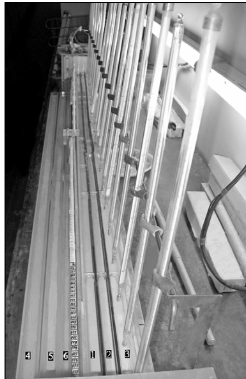
Fig. 1. Thermogradient apparatus: 1, 2, 3 – the sections of the gradient apparatus; 4, 5, 6 – the sections of the control tray
