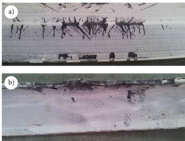
Fig.12. Failure modes and stress pattern in test specimens: a) flexural buckling; b) local buckling
