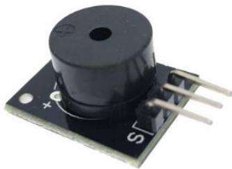
Gambar 7. KY-006 Passive Buzzer Module
