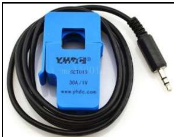
Figure 4. Current Sensors SCT013
