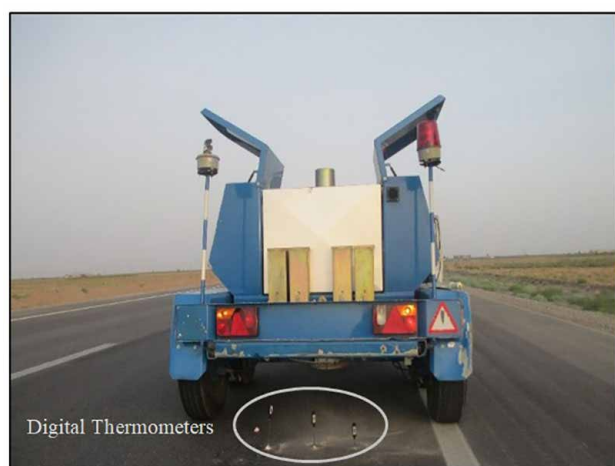
Figure 3. FWD testing and depth temperature measurements of asphalt layers on a pavement site
