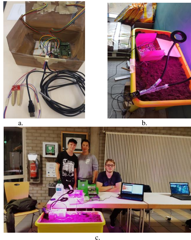
Figure 3: a. sensors to be put inside the plastic box field and their connection for senseBox, b. plastic box simulated as salad plants field filled with soil and necessary sensors connection, c. environmental setup for salad plant growth
