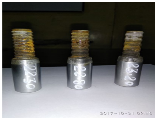
Fig. 3. Plug of sizes 22.30 mm, 22.80 mm, and 23.20 mm
