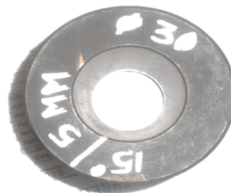
Fig. 2. Die of size 30.0 mm OD, 15 degree die semi angle and 5 mm land width
