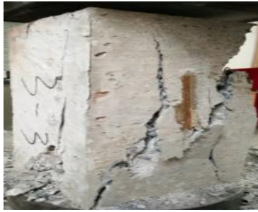
Fig. 3. Classic failure modes of test blocks with 50% of \delta and 4 kg/m 3 of m_{BF}
