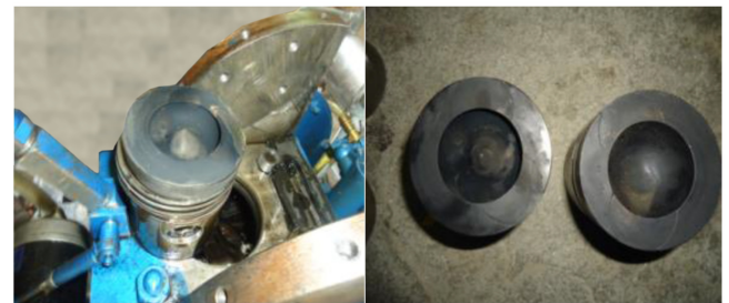
Fig.6. Photographic presentations of the piston disassembled after use.
