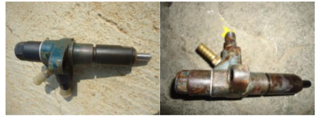
Fig.4. Photographic view of 3- and 5-hole nozzle fuel injectors.
