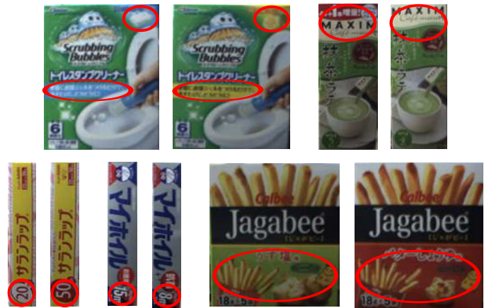
Fig. 8. Objects used in the experiment of recognition under occlusions. Red circles indicate the differences in color and/or texture between each pairs.
