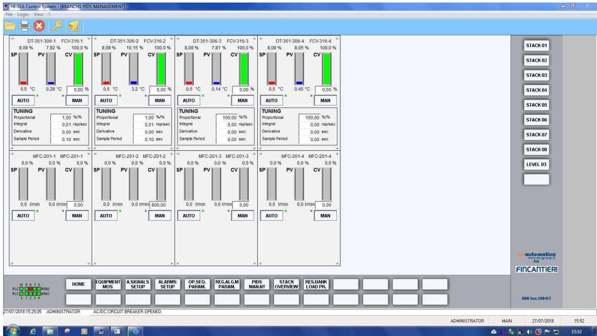
Figure 5.22 – HMI PIDS Management window
