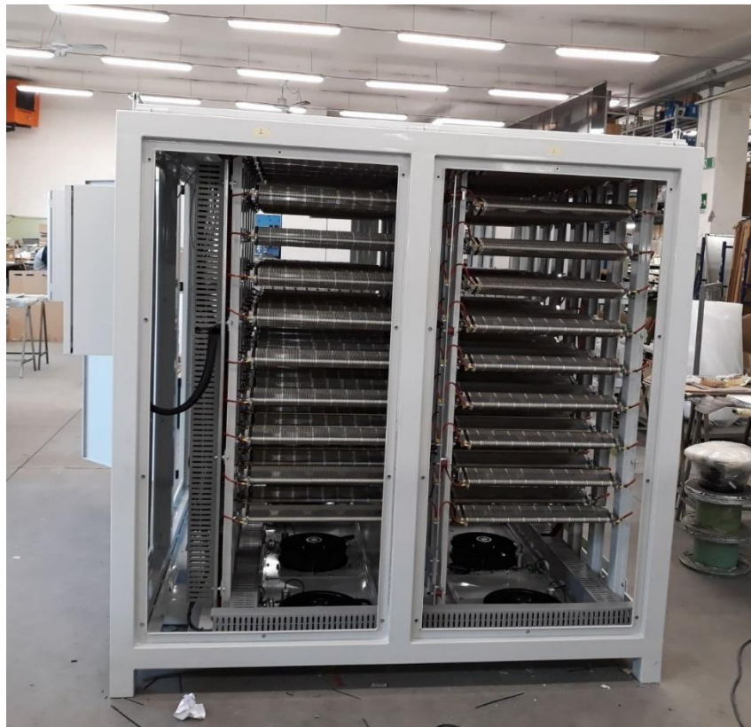
Figure 5.13 – SAE electrical load
