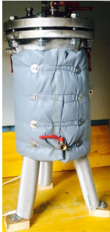
Fig. 2.1 Pilot scale STR, which can be used both in batch or continuous operation mode (Neviani et al., 2019).
