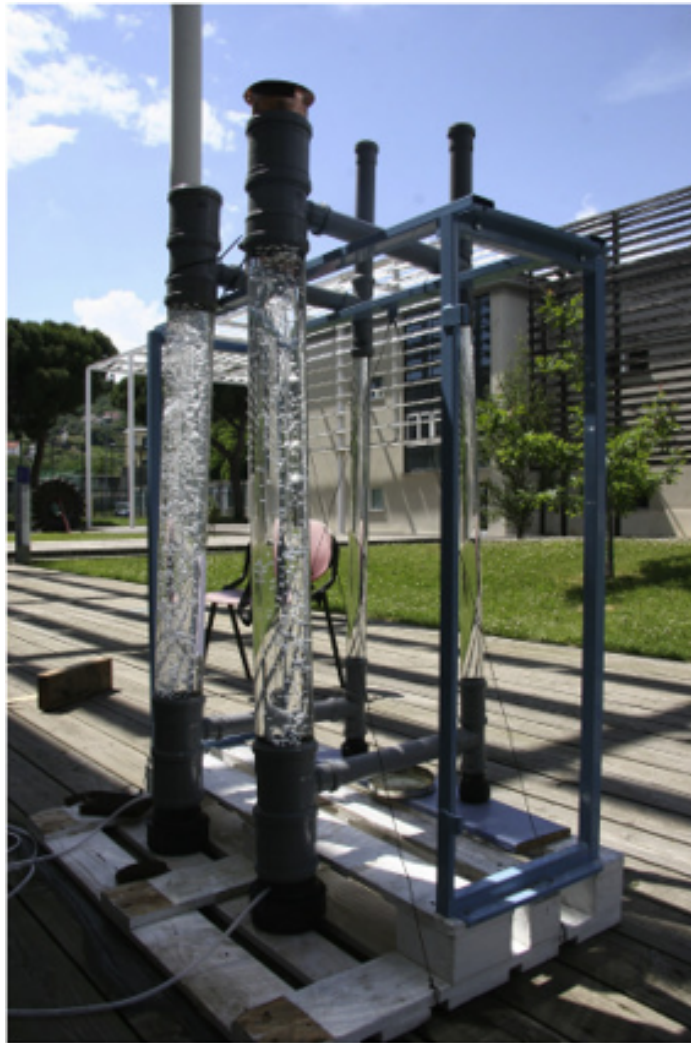
Fig. B.2 Two of the ALRs employed at pilot-scale (Paladino and Neviani, 2018).
