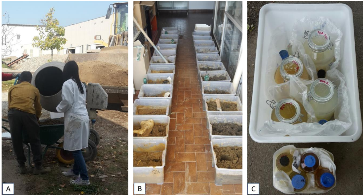
Fig. 1. A) Sample of artificially contaminated soil mixed in a cement mixer; B) Pilot-scale experiments with real polluted matrices; C) Mycological solution containing fungal inocula.
