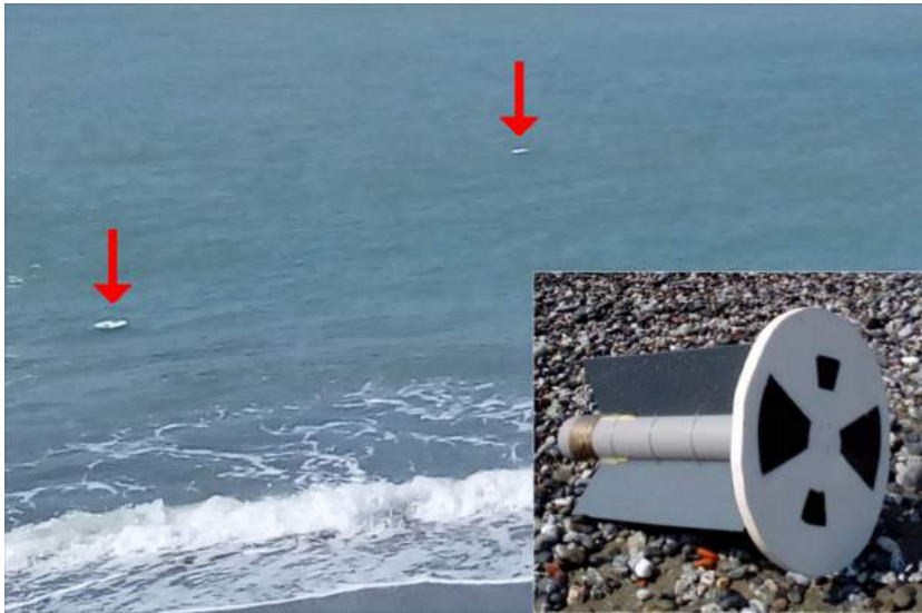
Figure 4.9: Design of the home-made drifters for the nearshore currents investigation.
