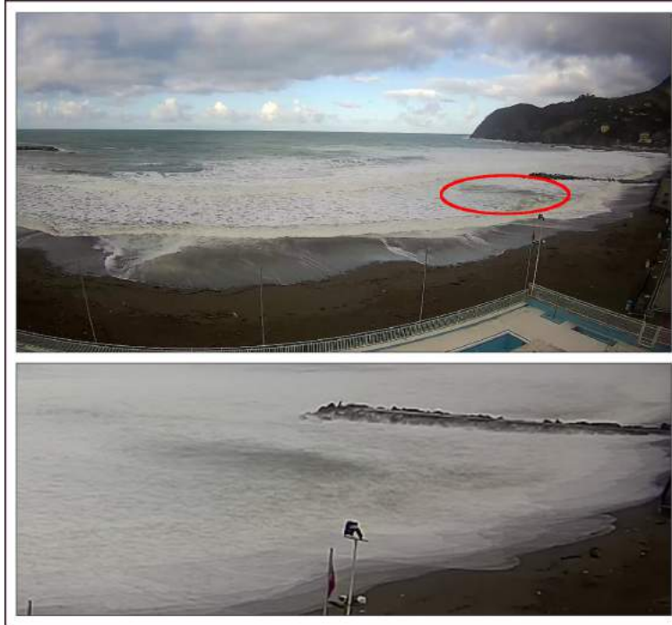
Figure 5.9: Figure 5.8: Rip current on the east side of groyne. (Top to bottom) snapshot image (rip current in red circle) and timex image (zoomed).
