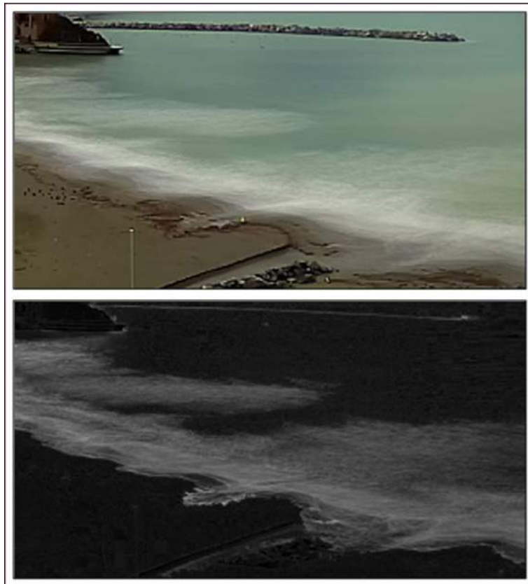
Figure 5.6: Rip current development in the central sector of beach eastern sector. (Top to bottom) timex and variance images.
