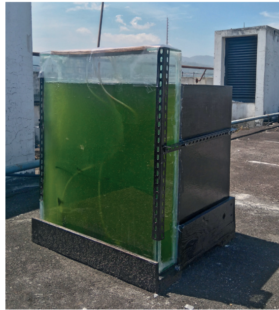
Fig. 5b. The application of algae photo-bioreactor in the building façade
