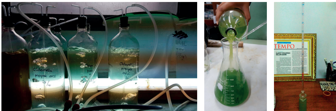
Fig. 9. The experiment to calculate Oxygen production from algae by using respirometer
