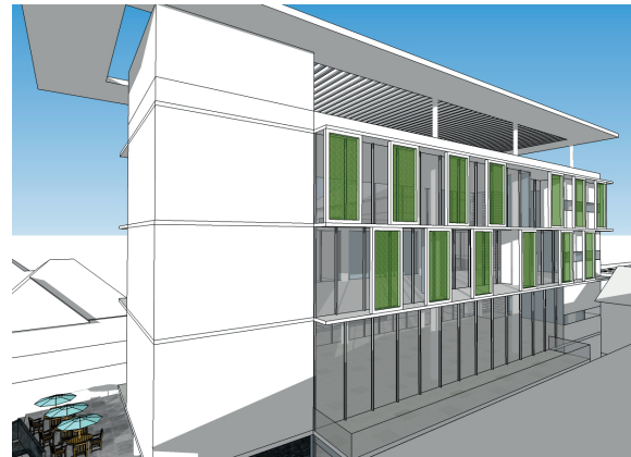
Fig. 4b. The application of algae photo-bioreactor in the building façade
