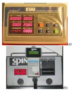
Figure 3: Emission detecting devices (a) Gas analyser (b) Smoke meter
