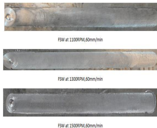
Figure 14: The appearance of upper surface of welding beads of 6061-T6AA plates produced by FSW.
