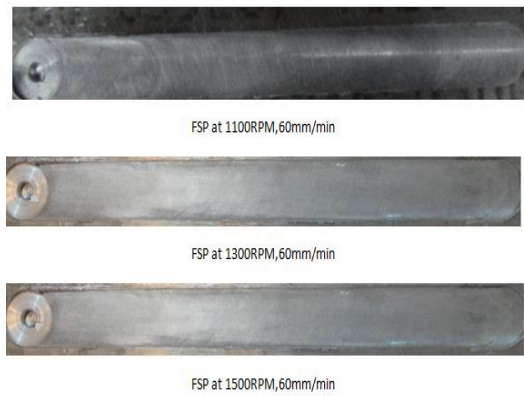
Figure 15: The appearance of upper surface of welding beads of 6061-T6AA plates produced by FSP.
