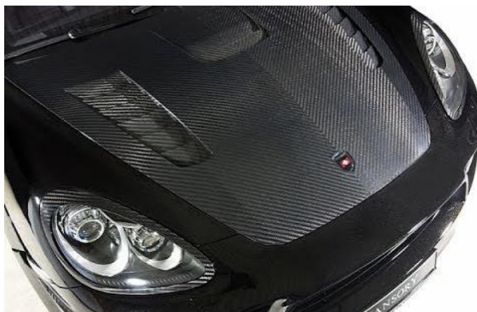
Fig. 4. Image of car bonnet made of carbon fiber [30].
