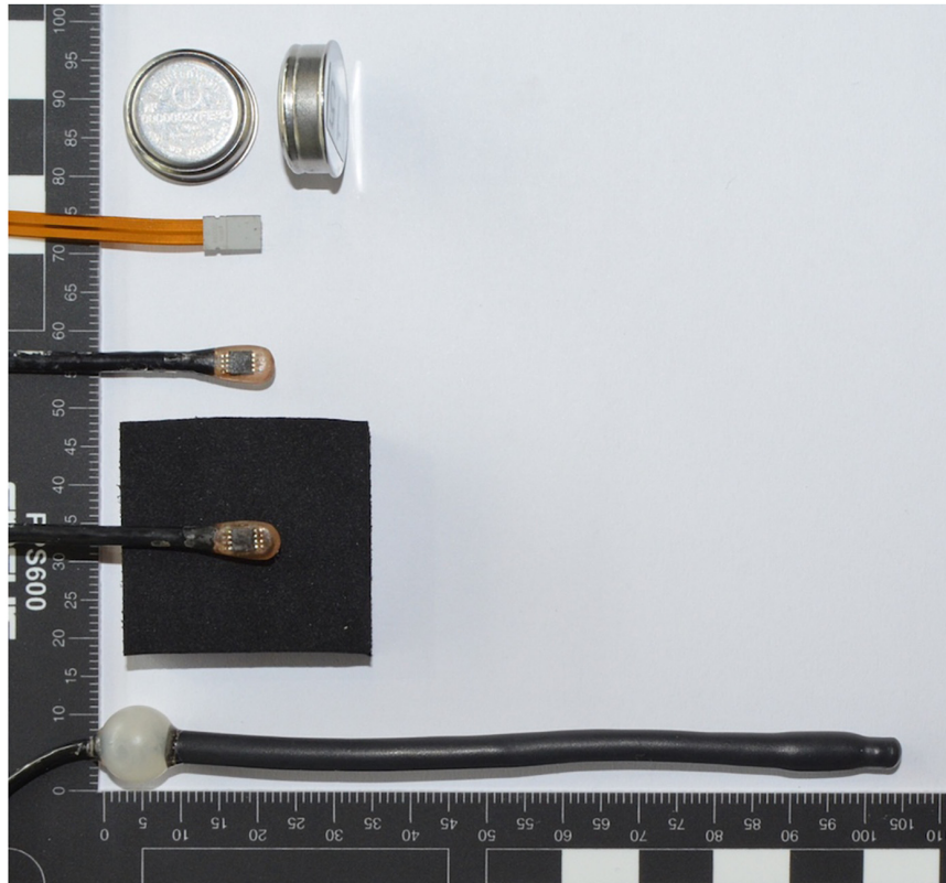
FIGURE 3 | Temperature and heat flux sensors used in the study (scale in mm). From top down: iButton, heat flux sensor, non-insulated temperature sensor, insulated temperature sensor (side in contact with the skin is facing upward), and rectal temperature sensor.
