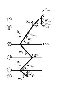
Figure 2 Reaction Force and Moment Analysis on Static Force System
