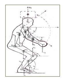
Figure 1 Model of Reaction Force and Moment Analysis on Static Force System
