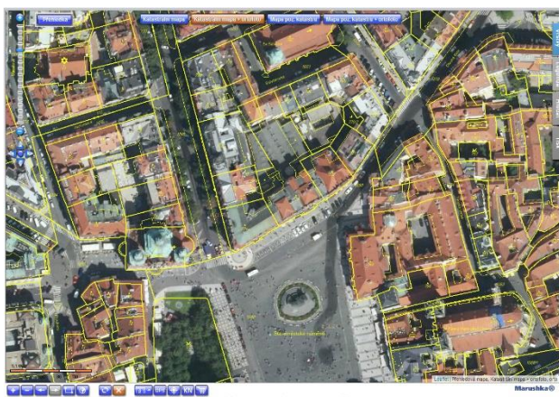
Figure 1. Cadastre map and orthophoto in web service by State Administration of Land Surveying and Cadastre. (ČÚZK, 2018)
