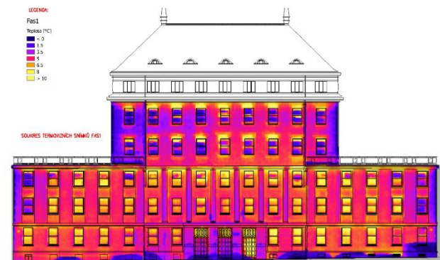
Figure 6. Thermal inspection layer included in MISYS SPRÁVA BUDOV.
