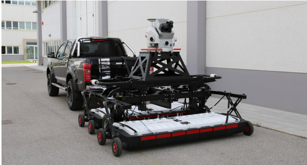
Figure 7. The IDS Pegasus:Stream combined above-ground and underground data capture platform is considered for a case study on mobile 3D GPR.
