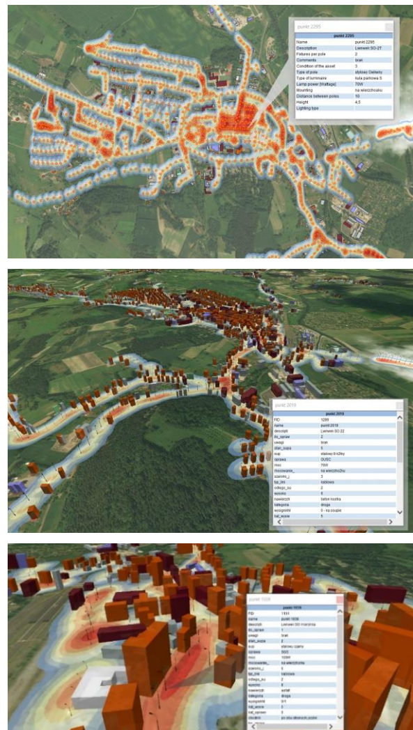
Figure 3. Example of a 2D and 3D access and visualization of the developed geodatabase for storing, querying and visualizing information of the street lighting inventory together with building models (LOD1) for the Municipality and Town of Lwówek Śląski (Poland).
