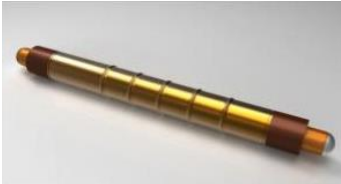
Fig. 8 - Geiger tube designed in CAD
