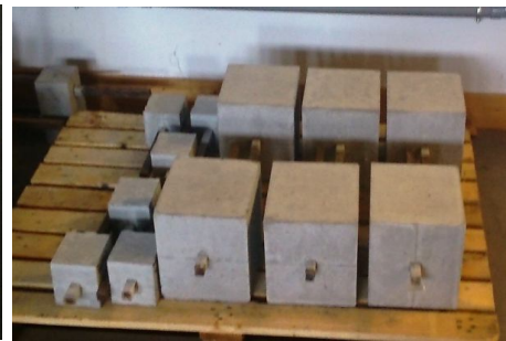
Picture 3. Pull-out specimen with 30 MPa of strength of concrete
