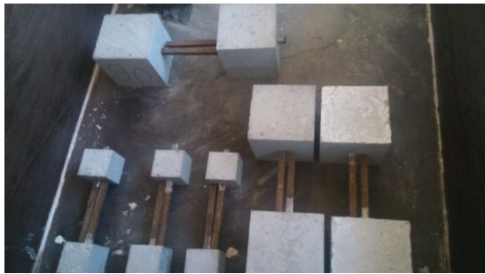
Picture 2. Pull-out specimen with 20 MPa of strength of concrete
