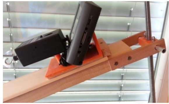
Figure 6. A spruce wood sample on an inclined tribometer made of spruce wood, detail of the load by the measuring device
