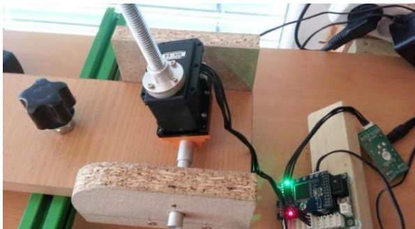
Figure 10. Detail of the setup of the measuring set for the precise detection of the moment, when during increasing/decreasing the elevation angle the body starts/stops moving over the friction surface
