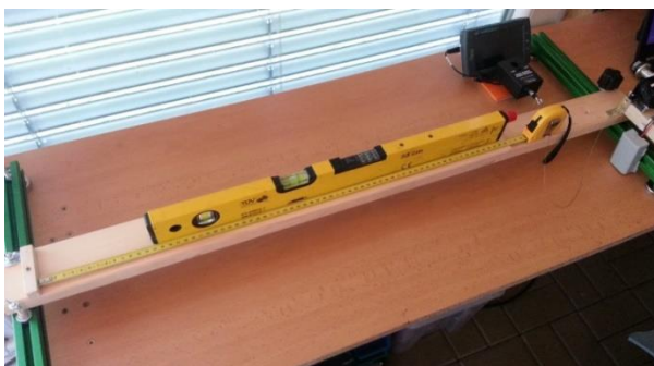
Figure 1. Friction bench for measuring the length of the contact surface (69.5 cm) its horizontal plane is established with the use of the libel
