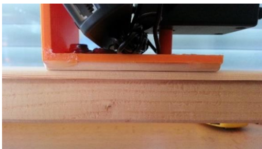
Figure 5. A spruce wood sample on a horizontal tribometer made of spruce wood, detail of the load by the measuring device
