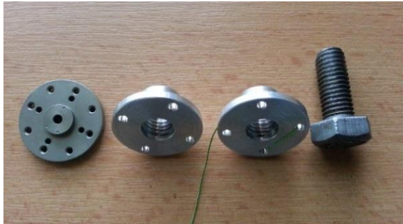
Figure 4. Dismantled external part of the composite shaft of the intelligent drive
