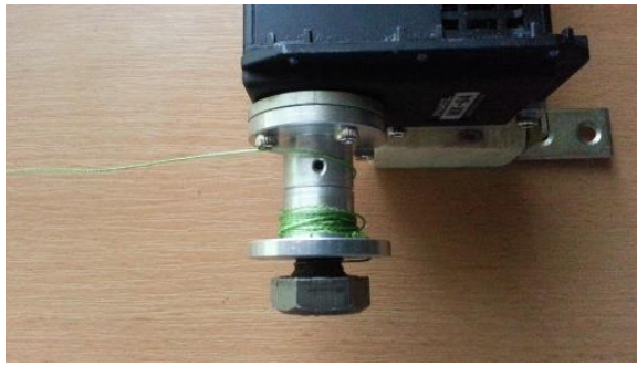
Figure 3. Self-manufactured external part of the composite shaft screwed onto the internal shaft of the intelligent drive
