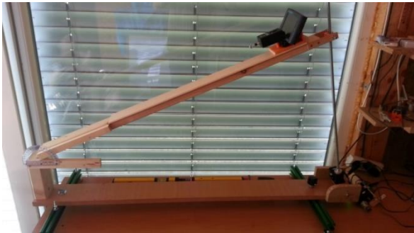
Figure 9. Friction bench arranged as a semi-automated inclinable tribometer
