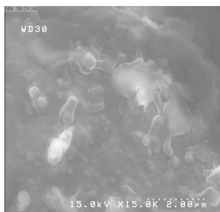
Figure 2: SEM image of the MWCNT-oil-based sample (with 1 vol.% MWCNT).
