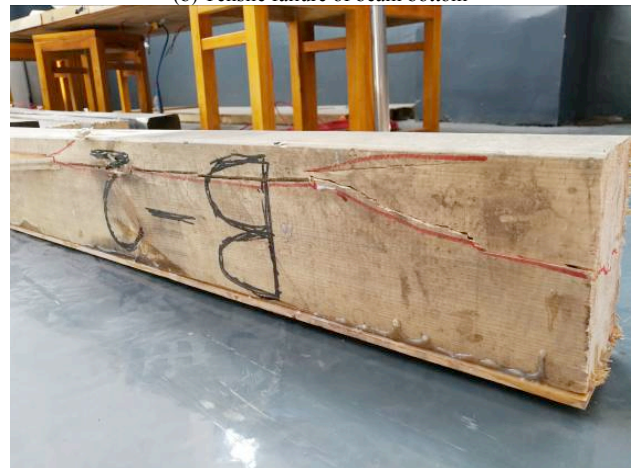
(c) Connected failure along the grain
