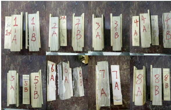
Fig. 3. Failure mode of bamboo-timber connection test specimens
