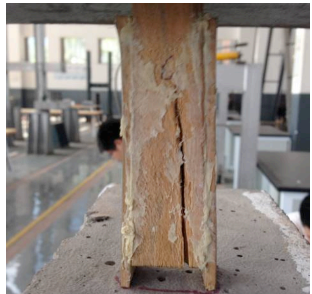
Fig. 2. Shear test of bamboo-timber connection specimens
