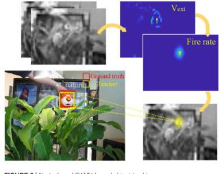
FIGURE 2 | Illustration of CANN-based object tracking.
