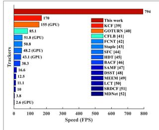
FIGURE 15 | Speed comparison with existing tracking algorithms (Danelljan et al., 2014a,b, 2015; Zhang et al., 2014; Galoogahi et al., 2015, 2017b; Henriques et al., 2015; Ma et al., 2015; Wang L. et al., 2015; Bertinetto et al., 2016a,b; Nam and Han, 2016; Qi et al., 2016). The data marked with "(GPU)" are tested on GPU while others are on CPU.
