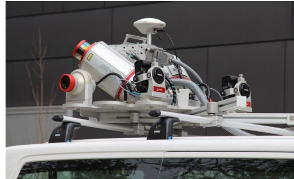
Figure 2: RIEGL VMX-250, mounted on a van
