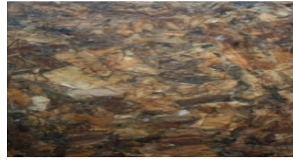
Gambar 2. Papan partikel dari kulit galam Figure 2. Particle board made from Galam bark
