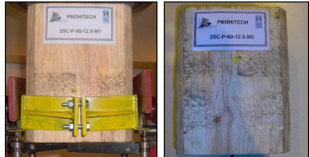
Fig. 24. Surface damage of the specimens without rubber layer
