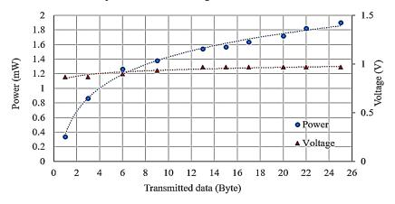
Fig. 9. Minimum power and voltage drawn by the proposed enhanced RF transmitter circuit during the active mode.
