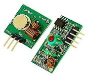
Fig. 2. RF wireless module used in this research, left transmitter, right receiver.
