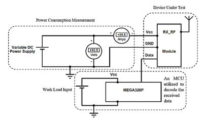
Fig. 12. Characterization circuit for RF Receiver.
