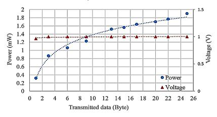
Fig. 6. Minimum power and voltage drawn by the conventional RF transmitter circuit during the active mode.
