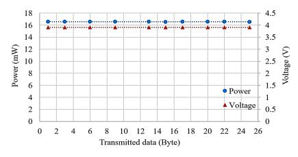
Fig. 13. Minimum power and voltage drawn by the RF receiver module.
