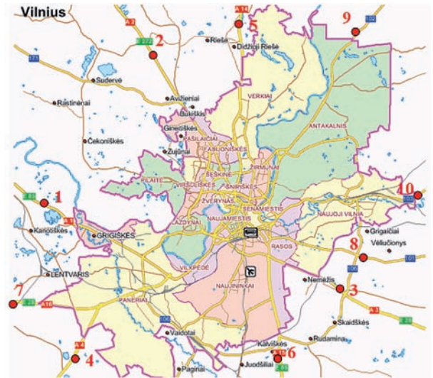
Fig. 3. Traffic intensity measurement posts installed on the roads of Vilnius region: 1 – road A1; 2 – road A2; 3 – road A3; 4 – road A4; 5 – road A14; 6 – road A15; 7 – road A16; 8 – road No. 101; 9 – road No. 102; 10 – Road No. 103 Lithuanian roads for the period 2000–2009
