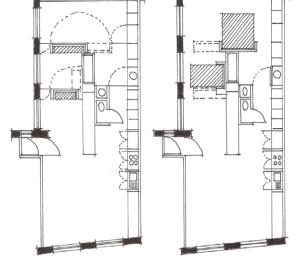
Figure 4. Embedding beds and other furniture in the walls as the edges of the rooms to allow multiple activities occur in the center, sample 33, 'The Transformable Apartment', Britain, 1996, Mark Guard Architects
