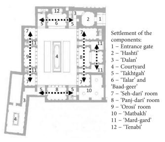
Figure 2. The soft Connection in the form of the portable thresholds in an inward-looking traditional Persian house, Sample 32 (Plan source: Ghezelbash & Abouzia, 1985, p. 23)
