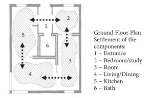
Figure 1. The soft Connection in the form of the portable walls in sample 27, 'Affordable Rural Housing', Britain, 2000, Architect: Gokay Deveci
