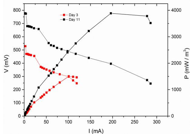
Fig. 2: Polarization curves of the MFC on the 3<sup>rd</sup> and 11<sup>th</sup> day using *B. cereus*.
