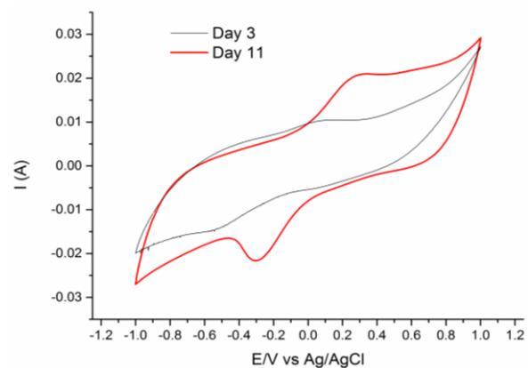
Fig. 5: Cyclic voltammetry curves of *B. cereus* on the 3<sup>rd</sup> day and 11<sup>th</sup> day of operations.
