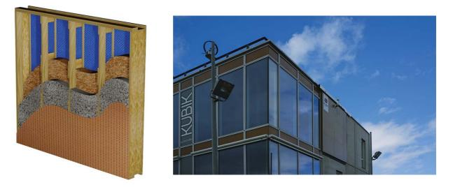
Fig. 5. Left: Scheme of the main elements composing the system; right: installed panel in Kubik.
