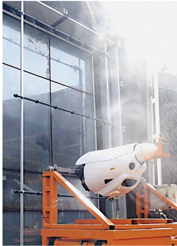
Fig. 2. Dynamic water penetration test for the fatigue process.
