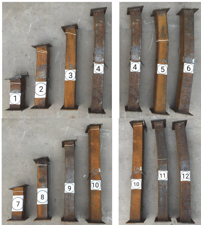
Figure 3: Failure forms of specimens.
