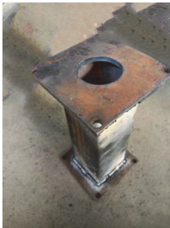
Figure 1: Specimen of the square steel tube.
