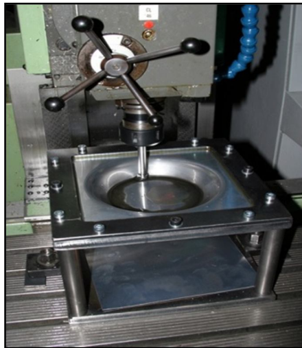
Fig. 1: Incremental sheet metal forming process [4].
