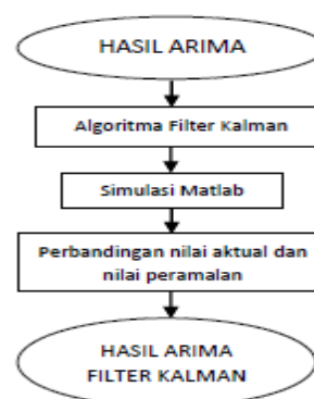
Gambar 2. Flowchart Kalman filter
