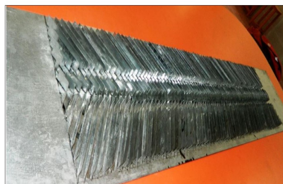
Fig. 35. Photographic view of discretized broken V-pattern baffle roughened plate [35].
